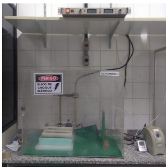
Figure 7. Conventional electrospinning equipment
