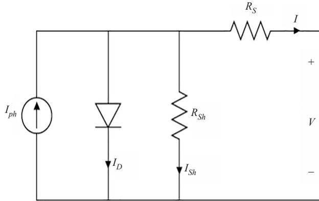
**Figure 1.** Equivalent circuit with shunt and series resistance
