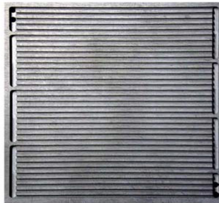
Figure 2. Micro serpentine bipolar flow plate [4]
