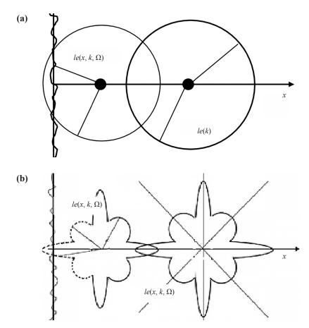
Figure 1. Explicit influence of the layer boundary on the mean free path of charge carriers and the associated relaxation length of fluxes with an isotropic distribution of properties (a) and with an anisotropic (conditional) distribution of properties (b) in a uniform thickness of a solid layer
