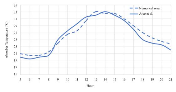
Figure 4. Comparison of solar chimney absorber temperature on October 9 between experimental results from reference [18] and simulated
