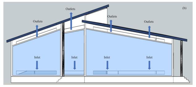
Figure 3. North view of the house designed in EnergyPlus, including walls and windows (a), South view of the house designed in EnergyPlus, which shows the solar chimney-The outside of the chimney is completely covered with glass to absorb most of the sunlight (b)
