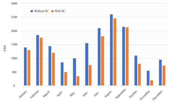
Figure 7. The amount of annual energy consumption in conditions with and without solar chimney for the city of Babol
