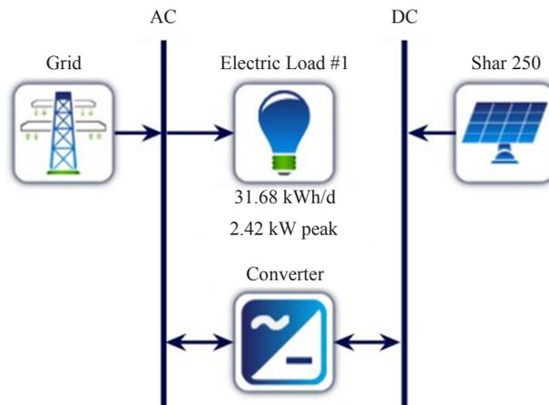
Figure 11. Design of building power supply system
