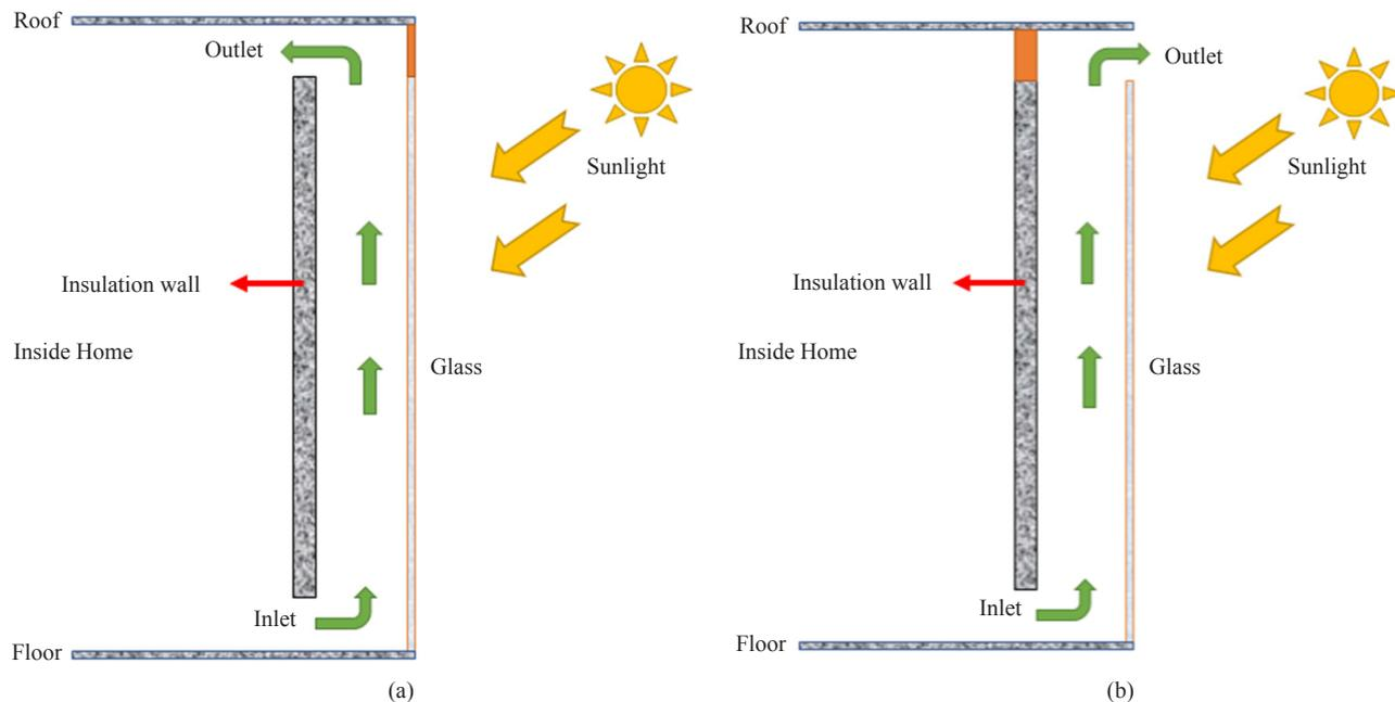
**Figure 1.** Two main types of solar chimney's operation: Winter SC-Passive heating mode (a), Summer SC-Natural ventilation and cooling mode (b)
