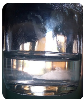
Figure 3. Image taken after incubation showing the formation of the biofilm on the surface of the pellet PA6/PL placed in contact with Enterococcus faecalis
