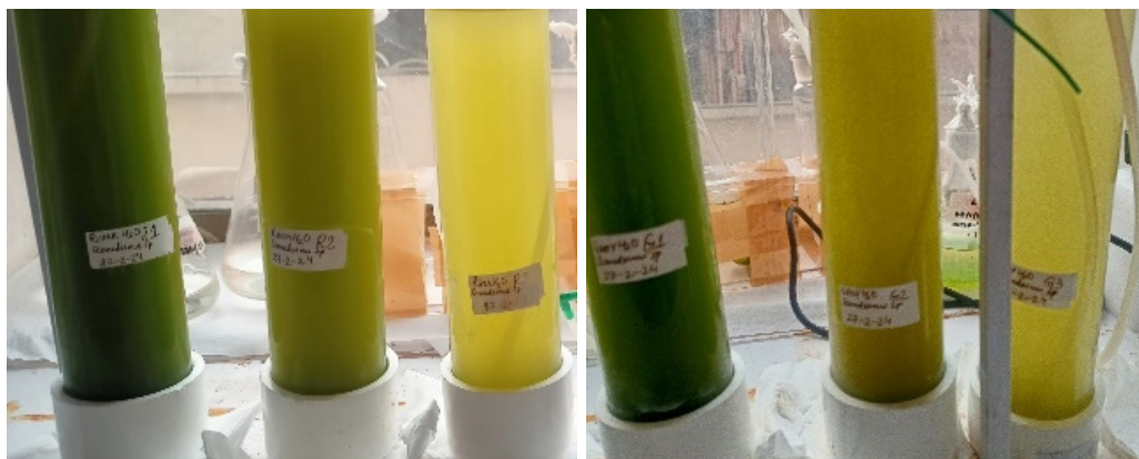
Figure 3. Microalgae culture tubes. From left to right: D. elegans grown in river water (R1)-supplemented only with N, P; (R2)-supplemented with 0.1X BG-11 medium; (R3)-control without any supplementation and in household grey water (G1)-supplemented only with N, P (G1); (G2)-supplemented with 0.1X BG-11 medium; (G3)-control without any supplementation
