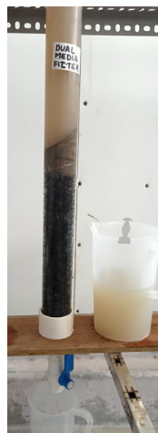
Figure 2. The domestic gray water with high turbidity (kept in the beaker) was run through the dual media filter composed of sand and activated charcoal
