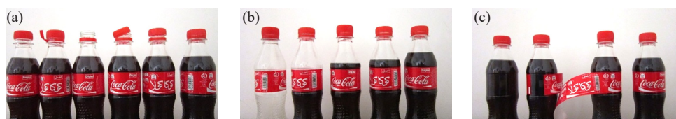
Figure 7. Common defects, (a) Cap, (b) Liquid level, (c) Label defects
