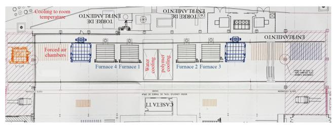
Figure 2. Heat treatment area layout
