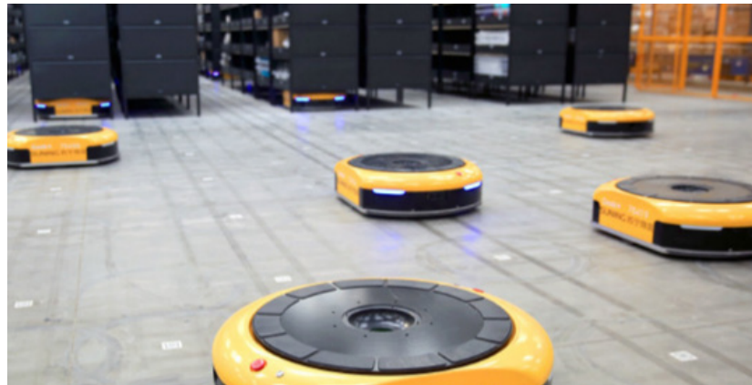
Figure 19. AGV for the automated conveyance of products and raw materials
