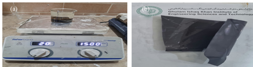
Figure 2. (a) Synthesis of STO@G/PVDF nanocomposite solution; (b) as-synthesized STO@G/PVDF nanocomposite film on a glass substrate
