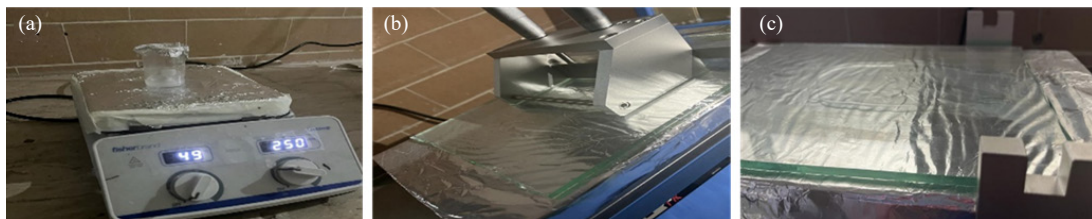
Figure 1. (a) Synthesis of PVDF solution; (b) automatic film coater equipment is used for the solution casting of the flexible polymer film; (c) as-synthesized PVDF film over a glass substrate
