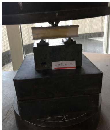
Figure 9. Flexural load setup
