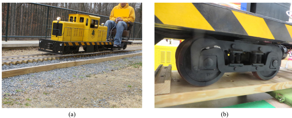
Figure 1. The electric MPM: (a) the MPMs; (b) fixed-axis bogie
