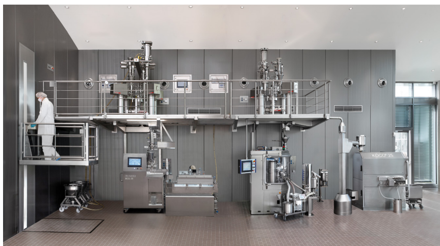
Figure 10. Example of a continuous tablet production line in an urban factory (photo reproduced with permission from © L.B. Bohle Maschinen und Verfahren GmbH).
