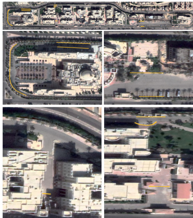
Figure 4. Proposed spots for rainwater collection catch basins
