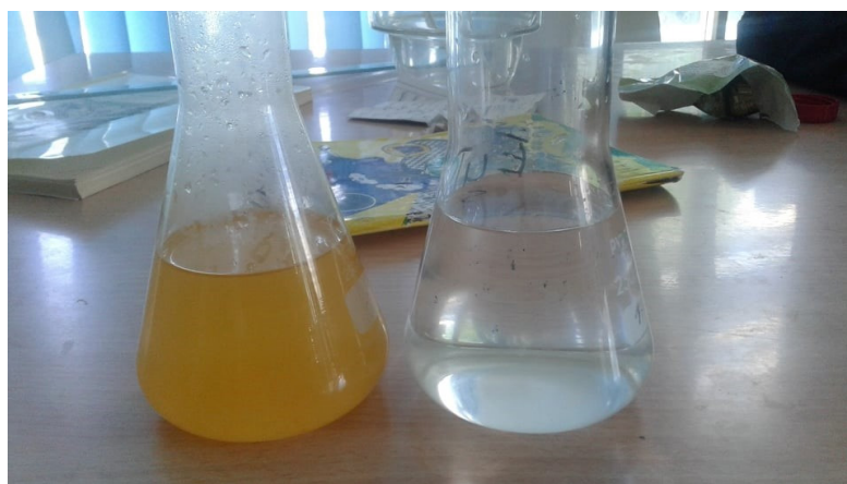
Figure 11. Membrane distillation treatment of rinse wastewater after steel pickling and treatment by precipitation-oxidation
