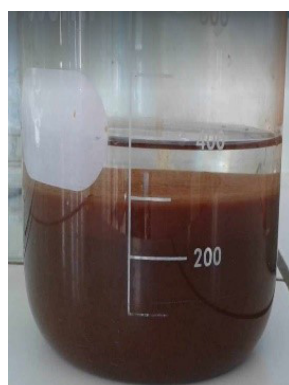
Figure 9. Sludge obtained after precipitation and oxidation of rinse water after steel pickling
