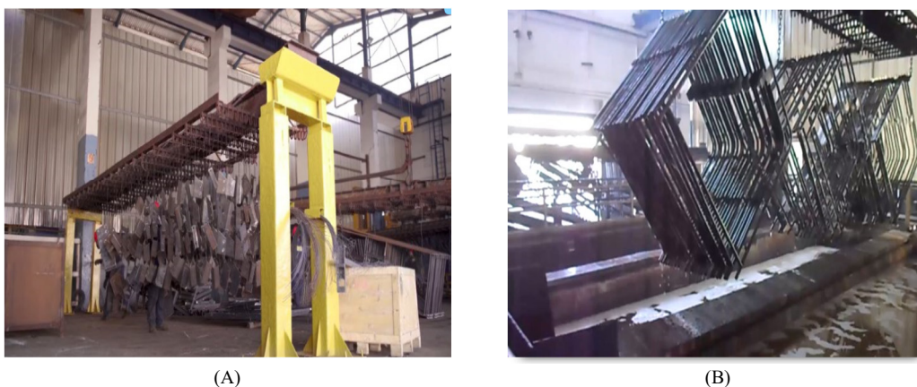
Figure 1. Photo of MBG-Galva steel galvanization steps; (A) hanging, (B) steel degreasing, pickling, and water rinse
