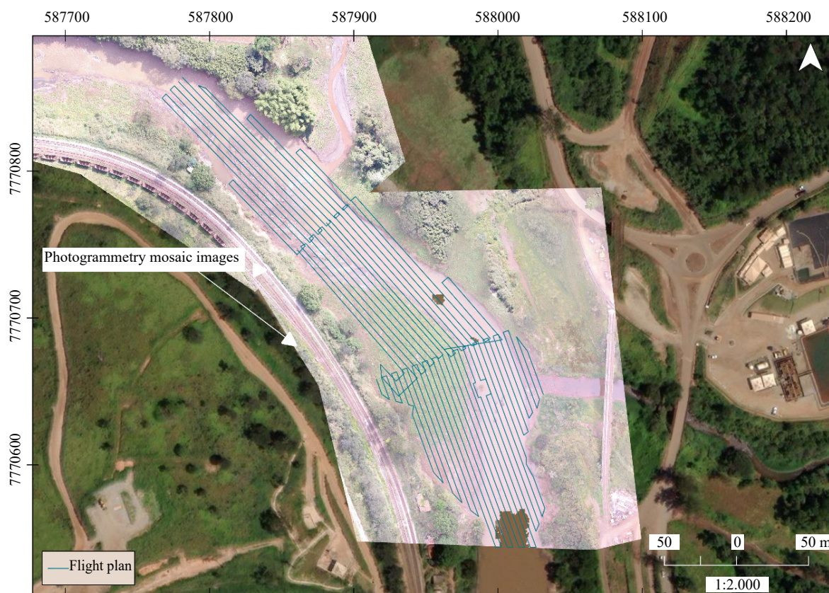
Figure 3. Example of the flight plans in the area known as “Ground Zero”
