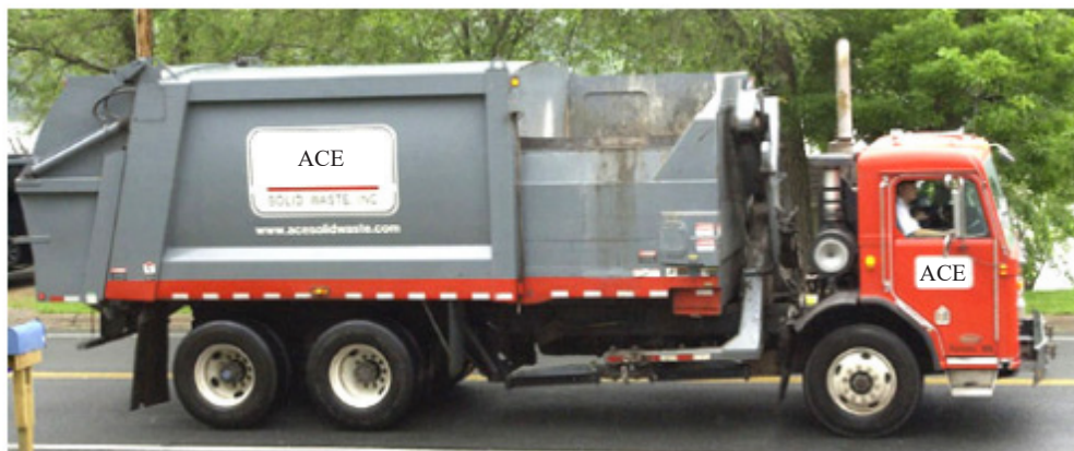
Figure 8. Refuse-truck duty cycle is the canonical application for hydraulic hybridization
