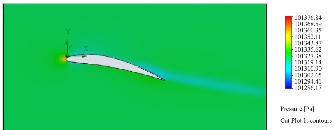
Figure 12. Pressure lineation to 30% dimpled aerofoil with 15° AOA
