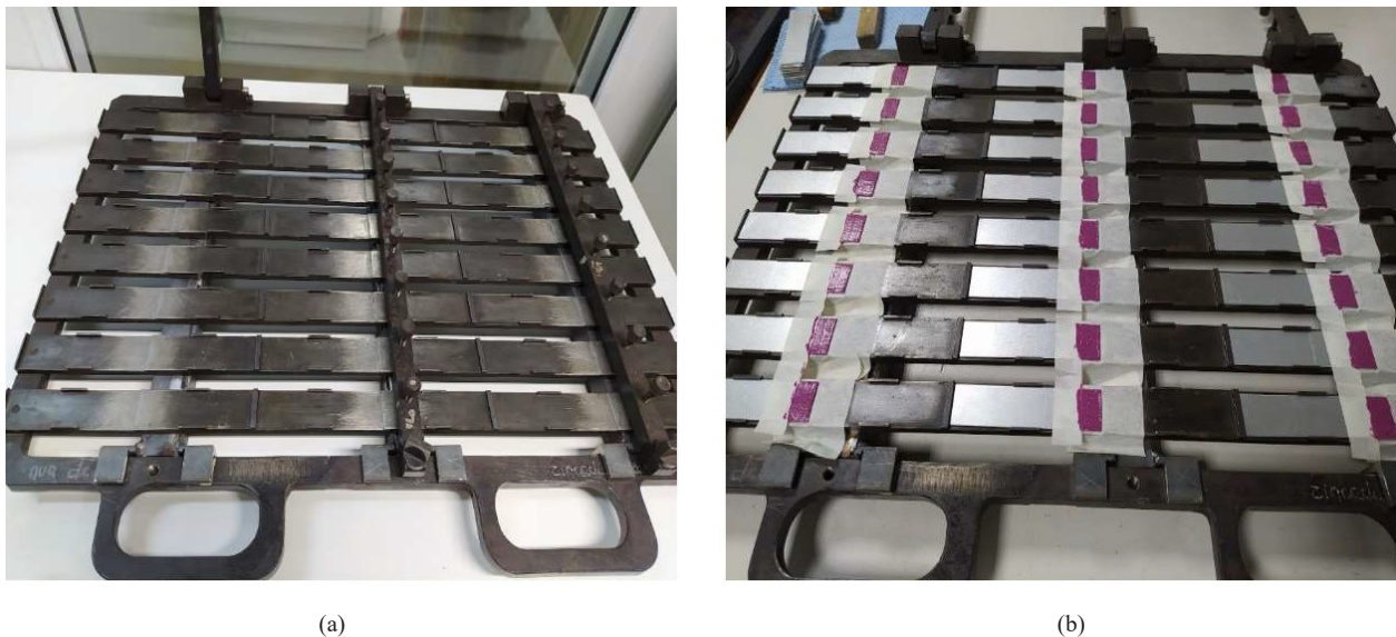
Figure 2. In-house device for single-lap joint preparation
