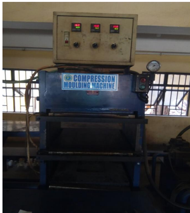
Figure 3. Compression moulding machine used for the composite formation
