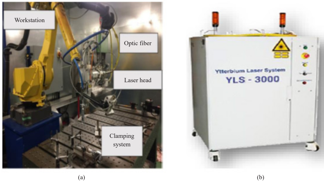
Figure 1. (a) Fanuc®M-710iC robot and HIGHYAG BIMO laser head (b) YLS-3000 laser source
