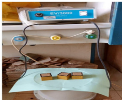
Poured geopolymer paste vibrated
