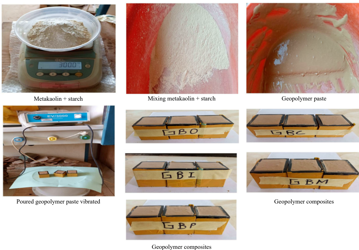
Figure 1. Mixing steps of the geopolymer composites
