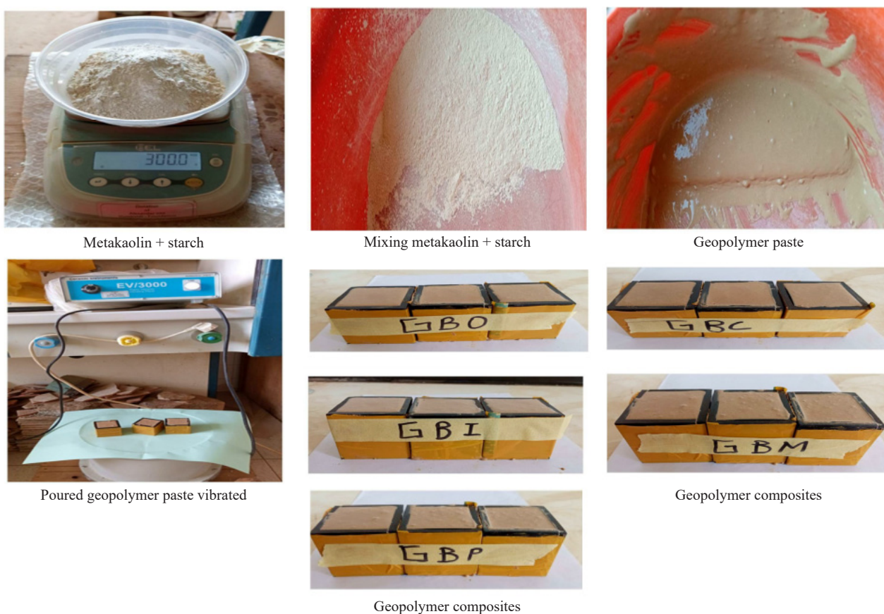
Figure 1. Mixing steps of the geopolymer composites
