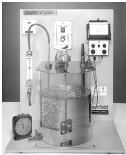
Figure 2. A typical bench-scale aeration unit (image from Armfield Ltd.)
