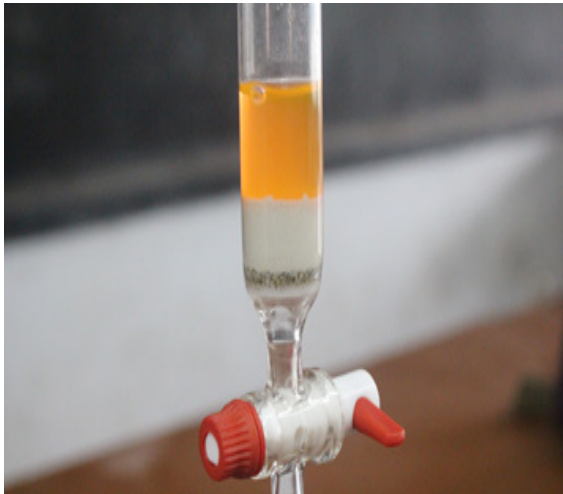
Figure 3. A column with a composite filter and dye solution
