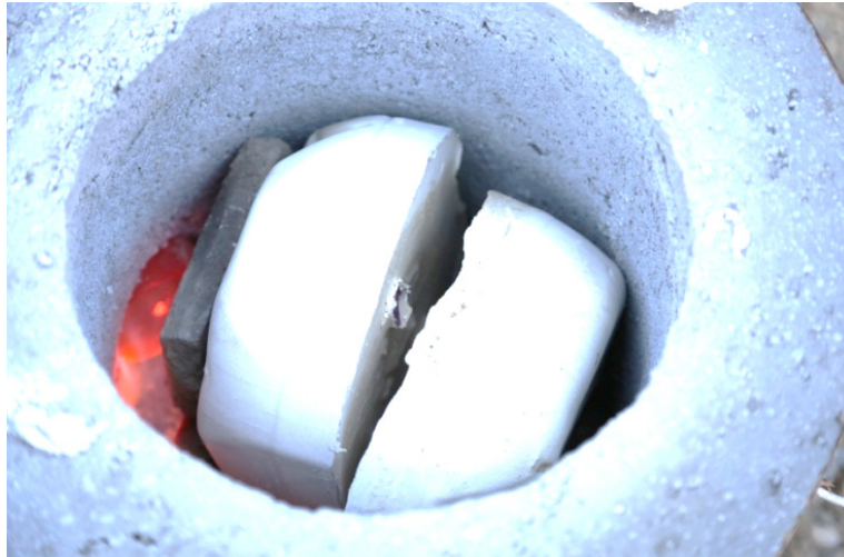
Figure 5. Burn out process
