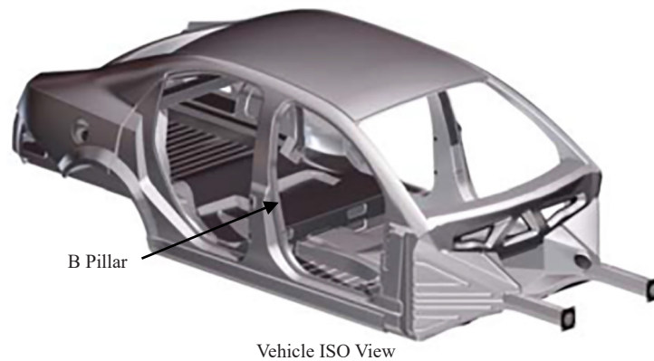
Figure 3. Standard vehicle-B Pillar design [2]
