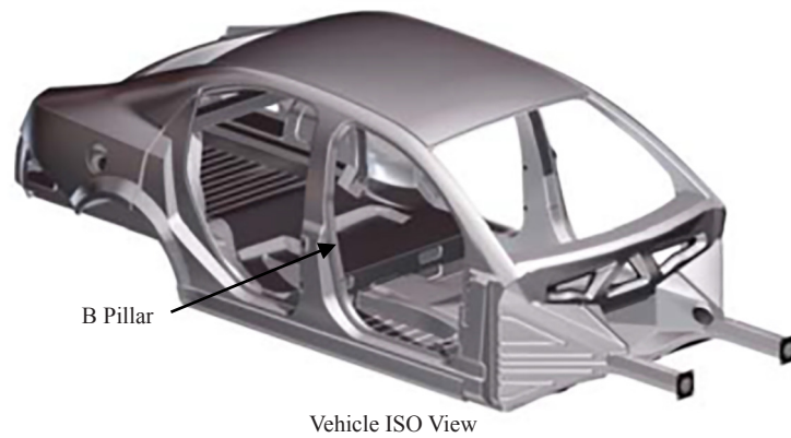
Figure 3. Standard vehicle-B Pillar design [2]
