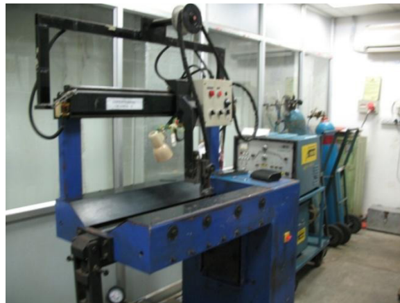
Figure 1. Micro Plasma Arc Welding setup
