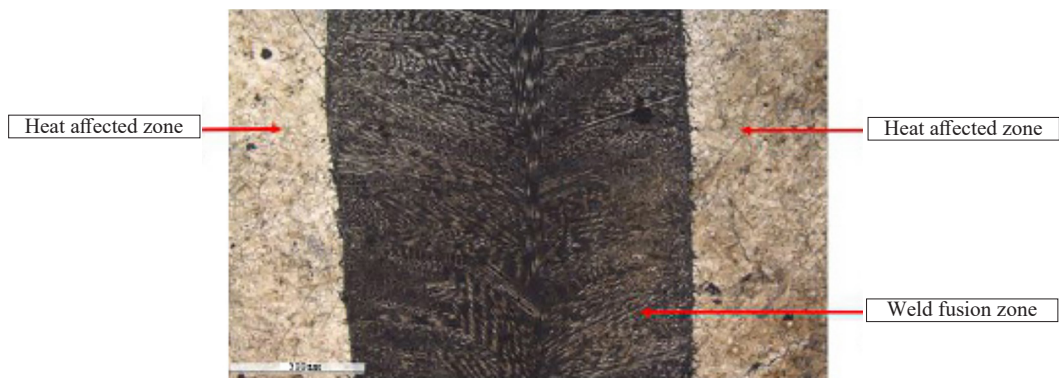
Figure 4. Microstructure of weld fusion zone and HAZ
