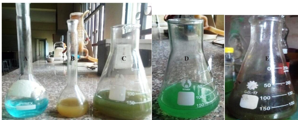
Figure 2. A: \text{CuSO}_4 \cdot 5\text{H}_2\text{O} , B: P. guajava extract, C: Before synthesis, D: P.g -CuNPs after synthesis at pH 5, E: P.g -CuNPs after synthesis at pH 8
