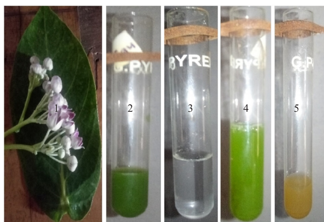
Figure 1. Sampling and stages in the preparation of the sample. 1: C. procera leaf and flowers, 2: C. procera extract, 3: Ampicillin solution, 4: Mixture before acid addition and heating, 5: Mixture after acid addition and heating
