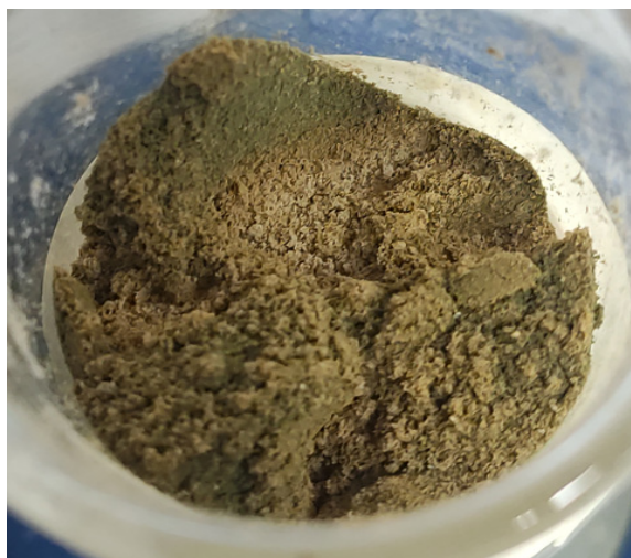
Figure 6. Mass of complex 11 after daylight exposure for about three weeks. Color changes from dark brown to khaki and partially green, as shown above
