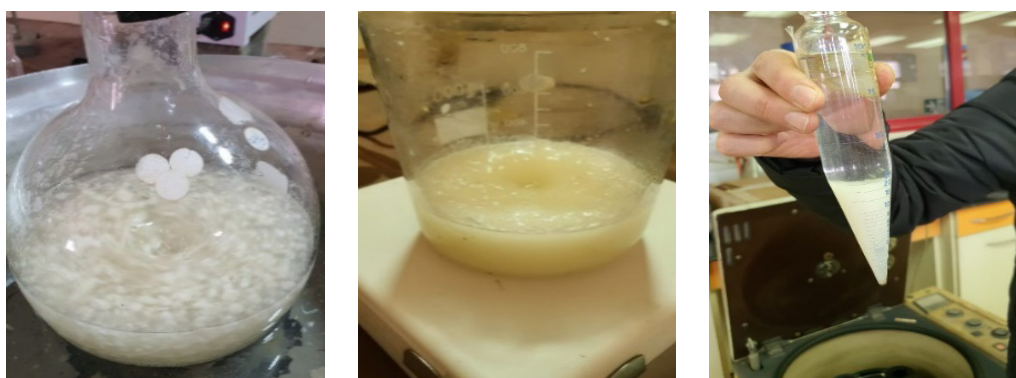
Figure 4. Preparation steps of cellulose nanocrystals
