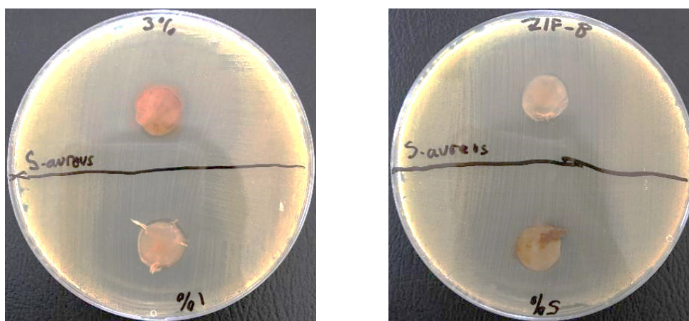
Figure 5. SCOBY immersion for 60 minutes in \text{Fe}_3\text{O}_4/\text{ZIF-8} solution with \text{Fe}_3\text{O}_4 concentration of 1, 3, 5% wt and ZIF-8 as a control against S. aureus
