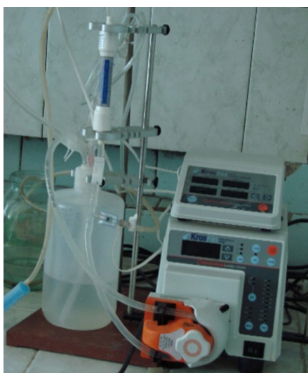
Figure 2. Krossflo DUF system
