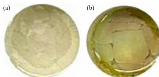
Figure 4. Visual comparison of lead borate glasses: undoped sample (a) and titania-doped sample (b), showing the noticeable color change induced by Ti addition
