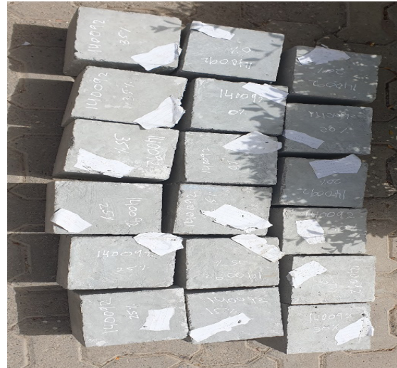
Figure 2. Completely dried concrete cubes
