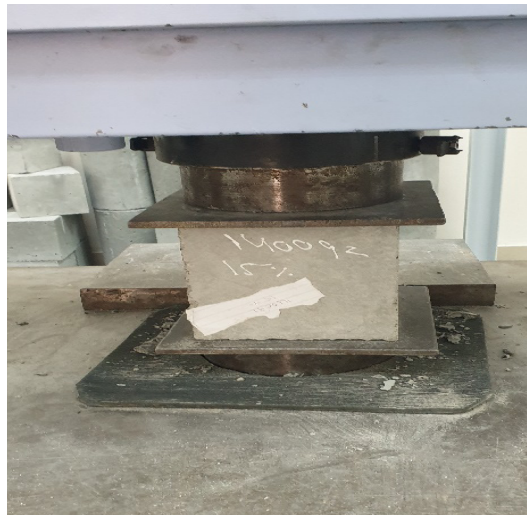
Figure 3. Compressive strength test on concrete
