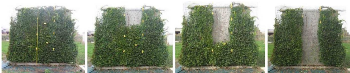
Figure 2. Direct LAI measurement process during the summer of 2013 [10]
