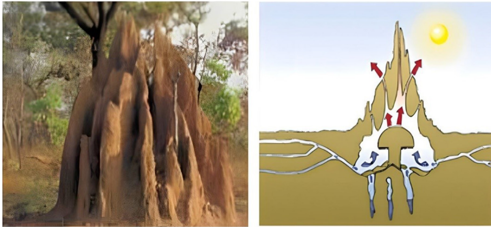
Figure 3. Termite mound and physiology working process as an inspiration for Council House 2 building [10]
