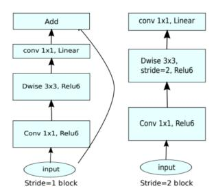
Figure 3. MobileNet-V2 architecture.
