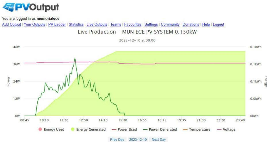
Figure 6. PV panel output power on Dec. 10, 2023, recorded in PVOutput.org.
