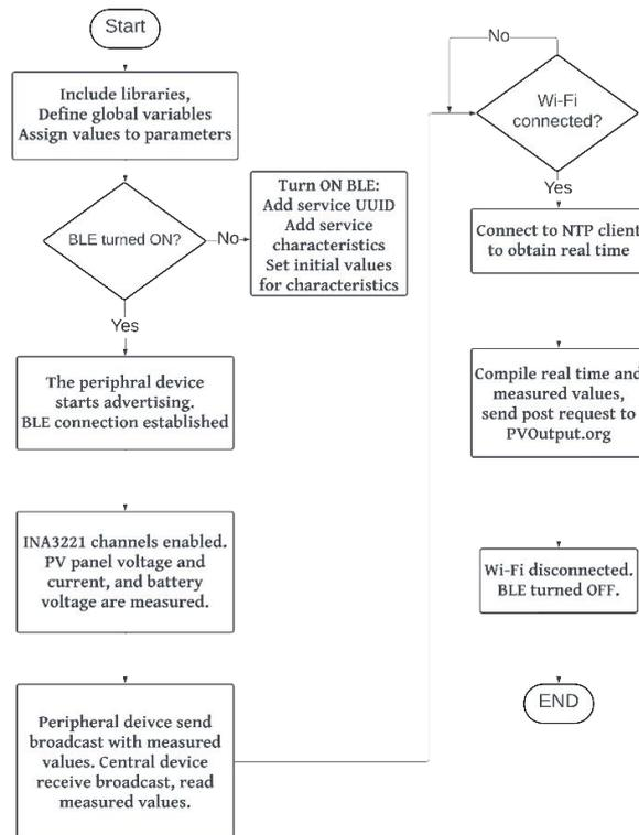
Figure 4. The SCADA system program flowchart.
