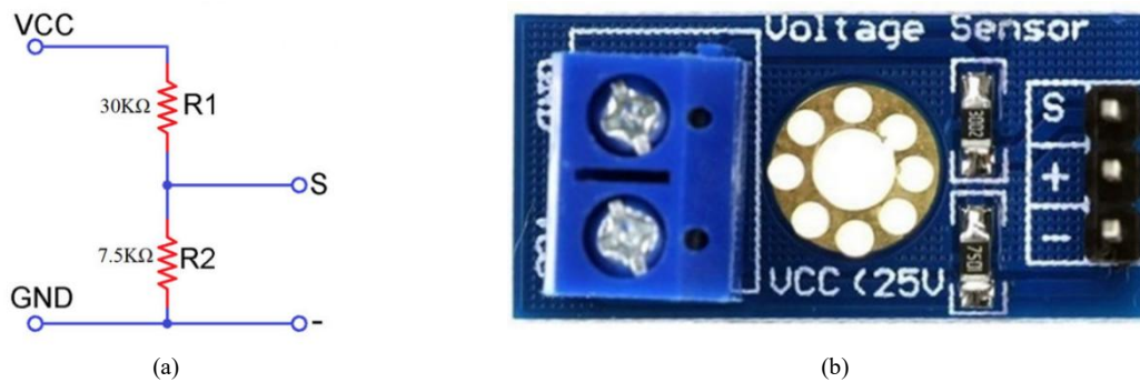
Figure 6. Voltage Sensor (0-25V). (a) Schematic Diagram. (b) Sensor Picture.
