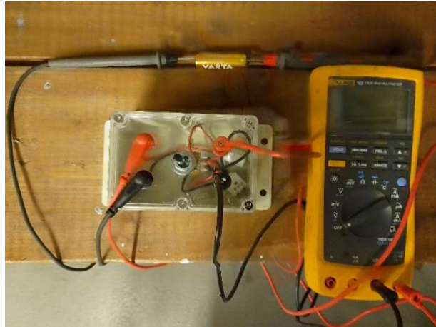
Figure 2. The battery's resistance measuring system. The lower red circle indicates an adjustable resistor (potentiometer). For the measurements, only specific boxes, certain measurement wires (red and black wires), and a reliable multimeter are required. The upper red circle marks the AA battery under test
