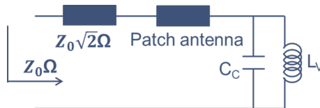
Figure 5. The equivalent circuit of the proposed antenna column.
