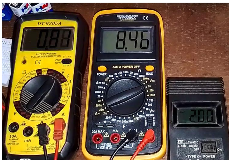
Figure 6. One of the reading screenshots for the reverse-biased IN5400 diode
