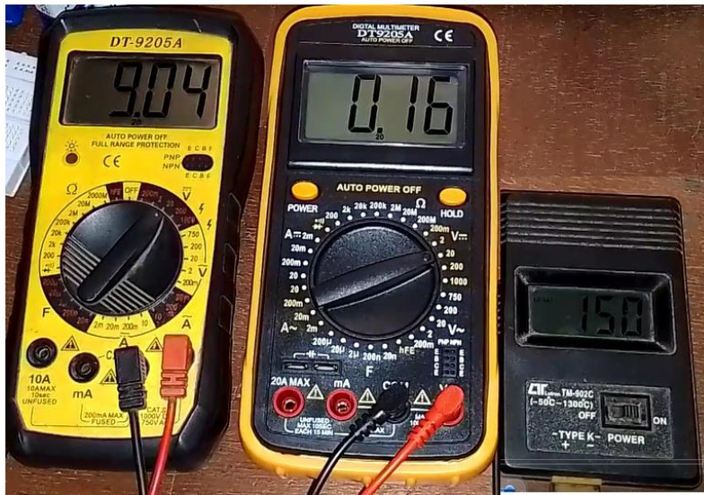
Figure 4. One of the reading screenshots for the forward-biased IN5400 diode
