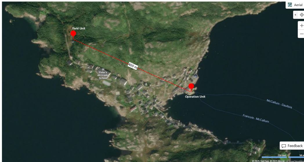
Figure 1. SCADA system with 400 m LoRa communication path in McCallum, NL, Canada [7]
