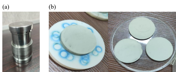
Figure 21. (a) PZT disk die; (b) Patches after pressing
