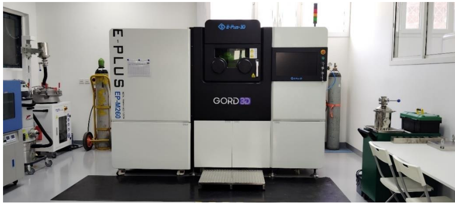
Figure 5. E-Plus-M260 Laser powder bed fusion machine
