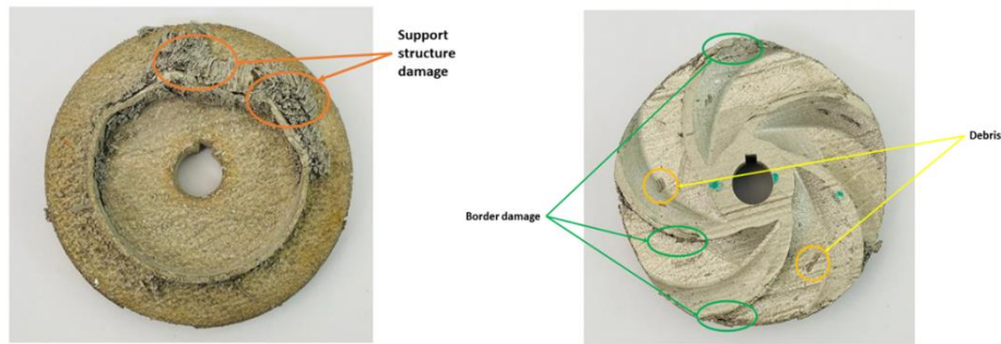
Figure 9. Support structure damage and debris for CI-D sample
