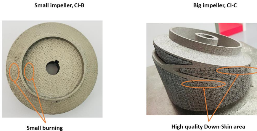
Figure 10. Impact of down-skin with big and small impeller with 30^\circ angle
