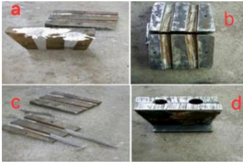
Figure 2. Fabrication procedure of AZ31 magnesium and eggshell-reinforced composite (a) Die with composite materials, b.) Open section of die, c.) Final composite materials, d.) A complete view of die)
