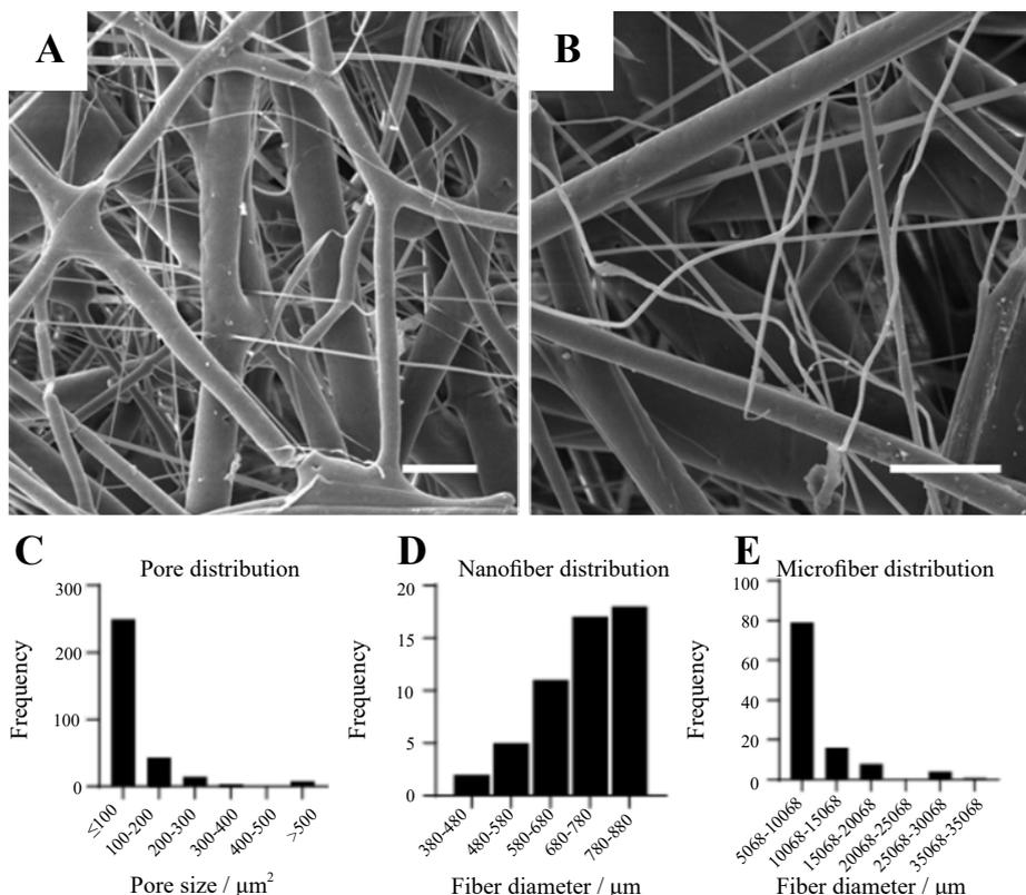
**Figure 2.** The process of melt-blown in combination with electrospinning, resulted in a micro/nanofibrous structure of the scaffold. The morphology of the scaffold was visualized using scanning electron microscopy (SEM). Magnification 3000 $\times$  (A) and 2000 $\times$  (B), scale 20  $\mu\text{m}$ . The histograms show distribution of pore size (C), nanofibers (D) and microfibers (E).
